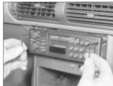
19.4 Withdraw the radio, using the tools to release the retaining clips
