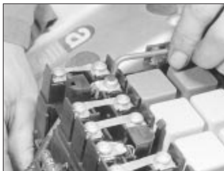
4.21b . . . undo the cable retaining screw . . .
