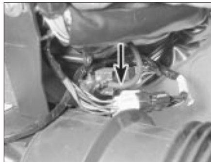
11.7 Solenoid vacuum hose (arrowed)
