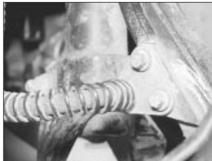
15.9 Front brake hose support bracket on the steering knuckle
