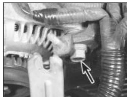
16.29a ... slacken the alternator side pivot bolt (arrowed) ...
