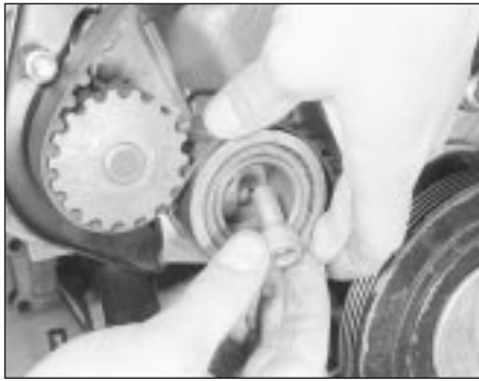
7.14 Removing the timing belt tensioner
