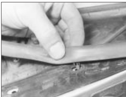
16.5b . . . and withdraw the sealing strip
