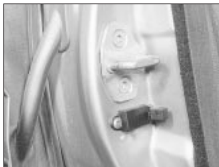
4.27 Courtesy light door pillar switch location
