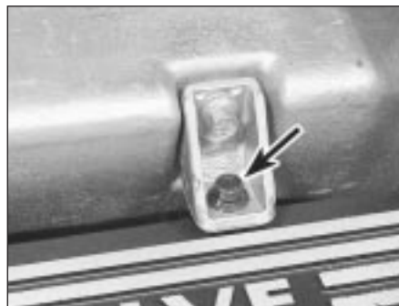
12.39 Plenum chamber mounting bracket to camshaft cover bolt (arrowed)
