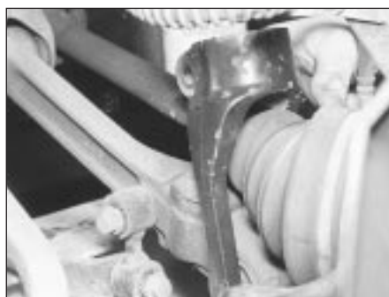
5.5 Removing the front suspension forked member
