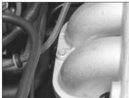
12.40 Plenum chamber to inlet manifold retaining bolt locations
