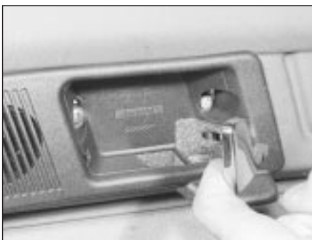
21.3b . . . and undo the trim surround screws
