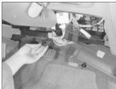
21.3b . . . and lower trim panel over the pedals
