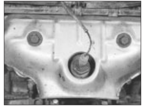
2.42 Rear oxygen sensor location in the exhaust manifold
