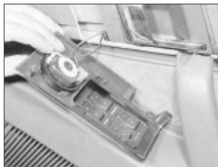
21.2b . . . and disconnect the tweeter speaker leads
