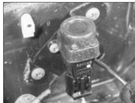
12.87 Inertia switch location on the engine compartment bulkhead
