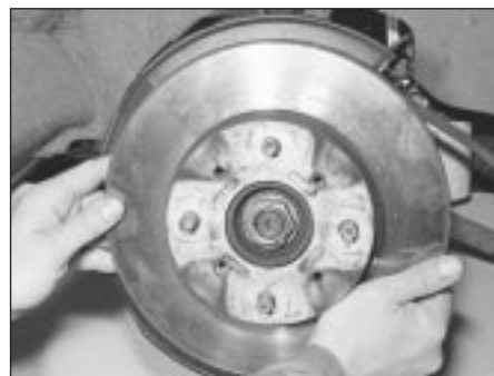
6.9b . . . and withdraw the disc from the hub flange
