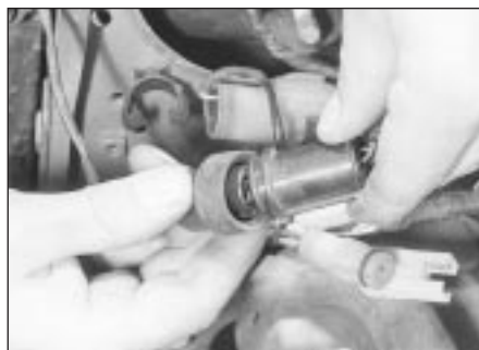
7.3 Separate the headlight main beam wiring at the connector
