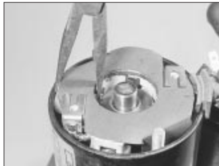
22.10 Using pointed-nose pliers to compress the brushes
