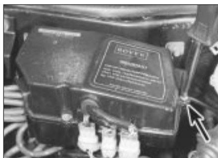
10.26 Undo the three screws and lift off the control box upper cover
