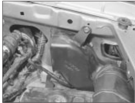
2.7 Side intake to body retaining bolt (arrowed)
