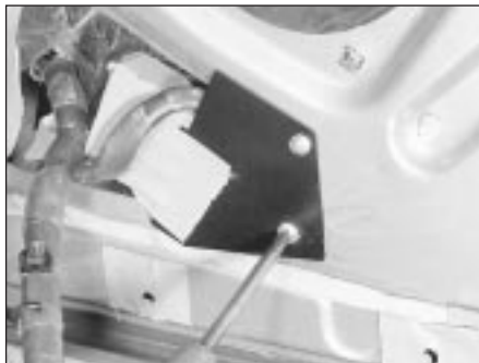
27.7 Undo the three screws and move the relay plate and relays aside
