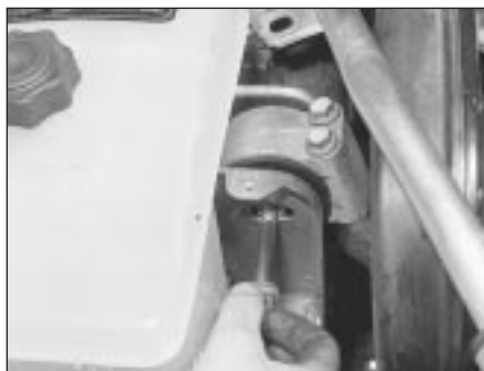
7.7 Undo the engine right-hand mounting through-bolt
