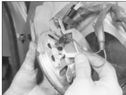
21.11 Withdraw the speaker and disconnect the wiring
