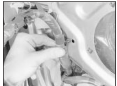
27.6b . . . and ease the loom away from the door
