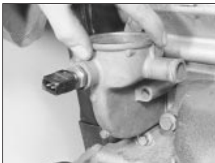
4.7 Removing the thermostat housing
