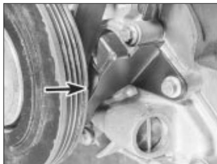
7.11c Crankshaft pulley timing notch (arrowed) aligned with timing belt bottom cover
