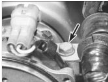
6.14 Undo the bolt (arrowed) and release the wiring harness from the side of the distributor body
