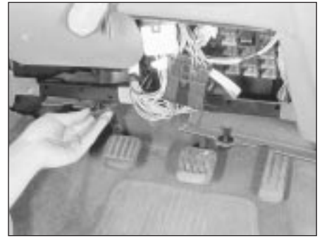
48.2 Remove the trim panel under the fascia
