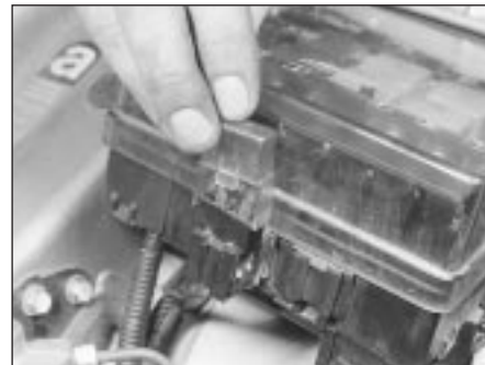
3.9 Additional fuse located under a cover on the outside of the fuse and relay box
