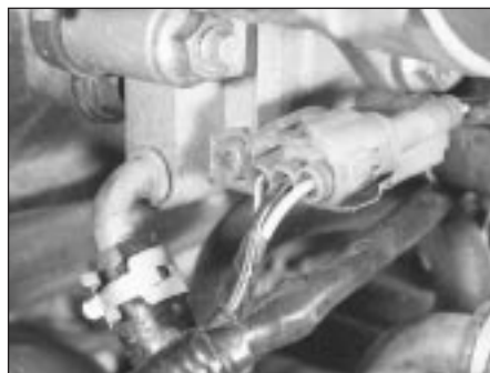
12.19 Throttle angle sensor wiring multiplug location
