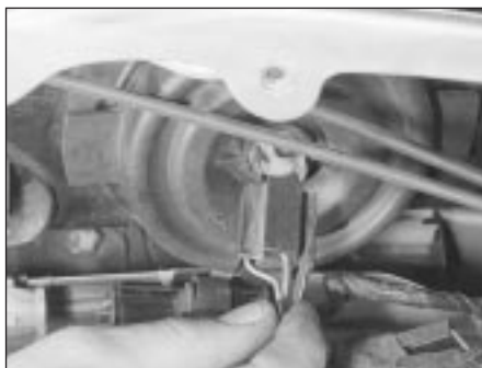
5.1 Disconnect the headlight dipped beam bulb multiplug
