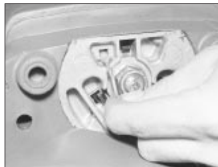
18.3b . . . and disconnect the two horn switch leads
