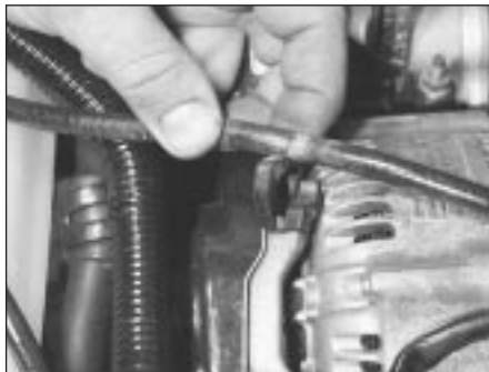
3.5 Release the cable from the support clips
