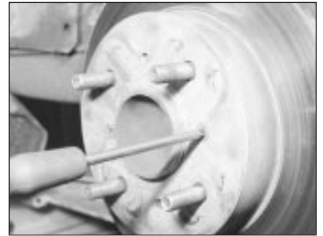
10.7a Undo the two retaining screws . . .
