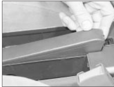
47.4 Prise up the handbrake lever cover trim
