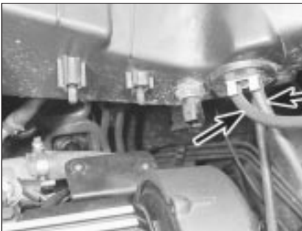
12.2 Thermac switch vacuum hoses (arrowed)
