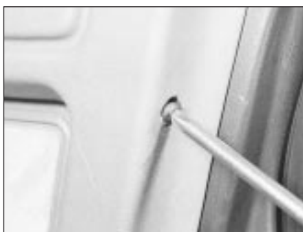
21.7b . . . and undo the recessed rear side screw
