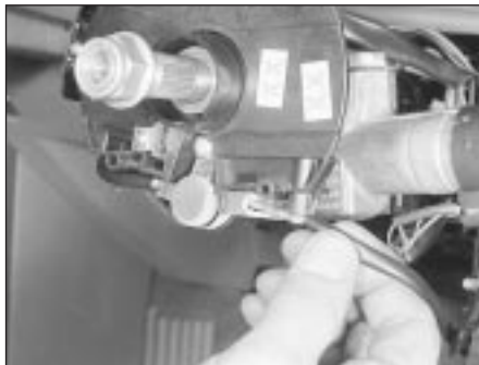
4.4 Release the fibre optic lead from the bulbholder
