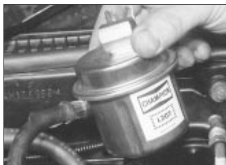
34.5 Undo the filter bracket retaining nuts or bolts, and remove the filter
