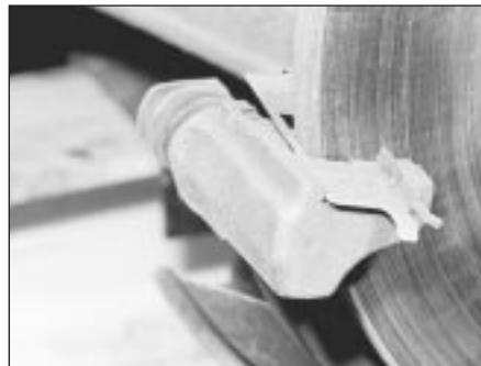
7.6c ... and lower anti-rattle shim
