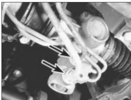
24.10 Unscrew the two fluid pipe union nuts (arrowed)
