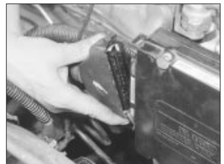
12.47 Disconnect the ECU wiring multiplug
