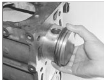
11.6 Removing the piston and connecting rod assembly
