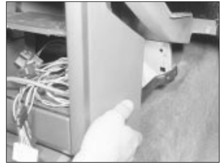
48.11b . . . and remove the lower facia
