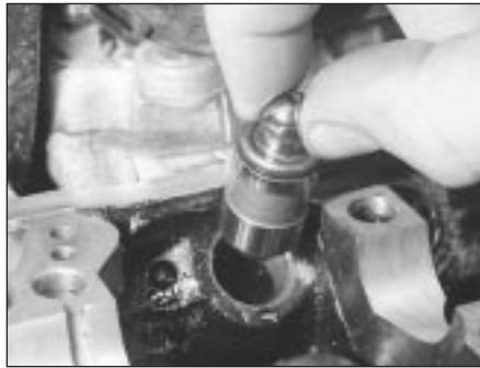
15.16b . . . and hydraulic tappets
