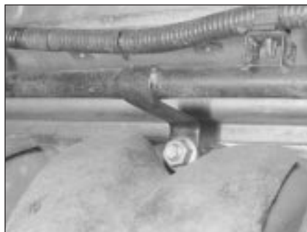
6.11 Undo the manifold nuts and bolts, noting that the upper nut also secures the bypass pipe bracket
