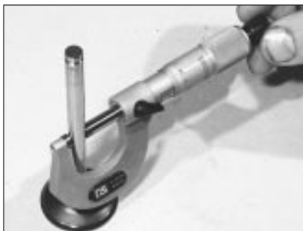
9.12 Measuring the valve stem diameter
