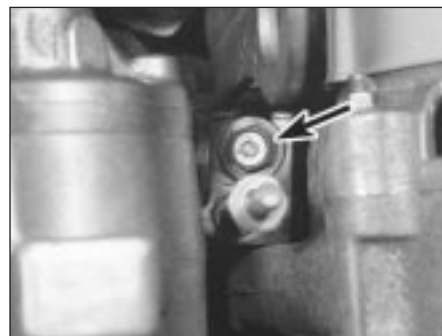
17.10b . . . and adjusting bolt (arrowed)
