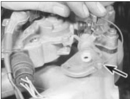
3.3 ... and release the cable end (arrowed) from the throttle cam
