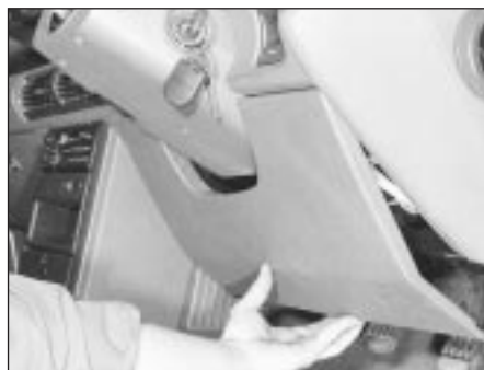
21.3a Remove the upper trim panel . . .
