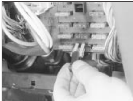
3.3b . . . to withdraw the fuses from their locations
