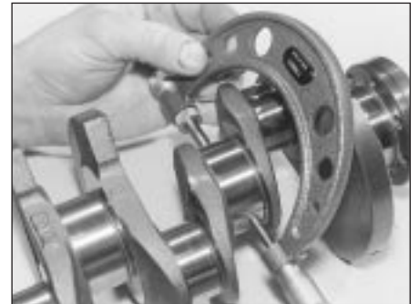
17.4 Measuring the main bearing journal diameters
