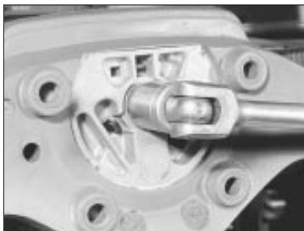
18.6 Undo the steering wheel retaining nut
