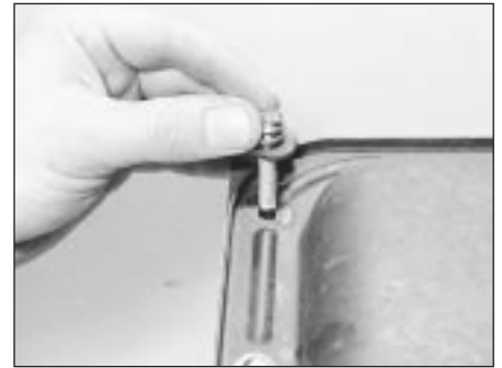
13.8 Sump special retaining bolt location
