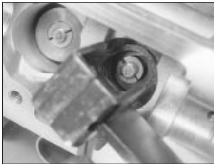
7.2 Compress the valve springs with a universal valve spring compressor
