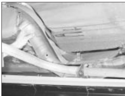
20.3 Removing the rear heat shield from the exhaust system
