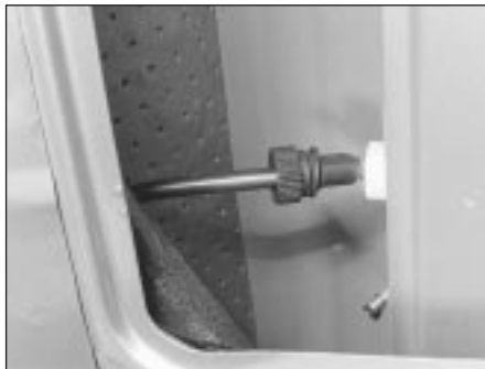
5.33 Number plate light bulbholder on early Saloon
