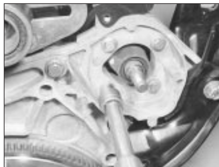
26.15 Undo the four pump retaining bolts
