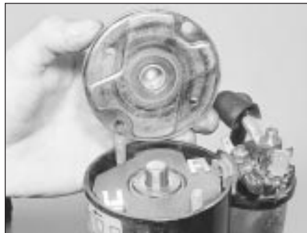
22.3 Withdraw the commutator end bracket
