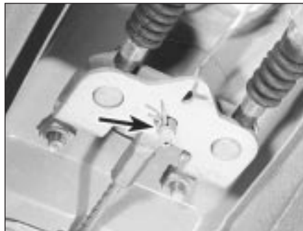
19.4 Extract the cable retaining spring clip and clevis pin (arrowed)
