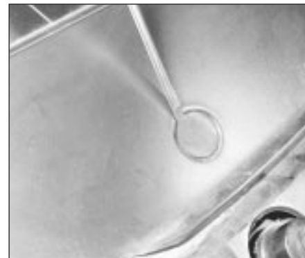
16.3 Prise up the windscreen finisher screw caps
