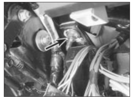
21.10 Steering column upper mounting nut (arrowed)
