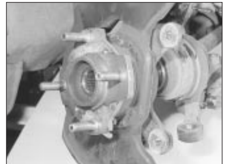
2.13 Withdrawing the steering knuckle from the driveshaft
