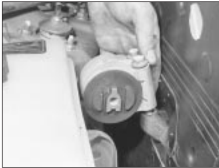
4.43 Remove the right-hand engine mounting
