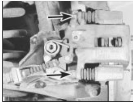
7.4 Rear caliper upper and lower guide pin bolt locations (arrowed)
