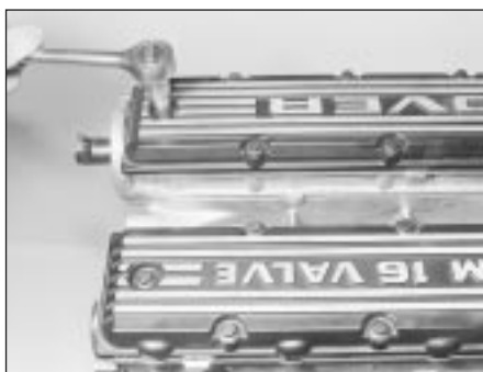
4.4a Undo the camshaft cover retaining bolts . . .
