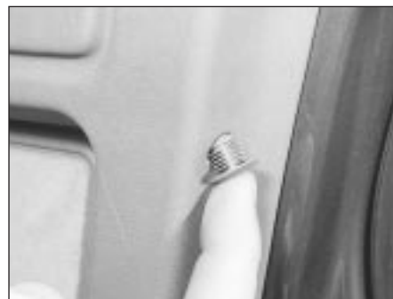
21.7a Pull out the blanking plug . . .
