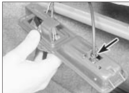
44.3 Extract the outer cable retaining clip (arrowed) at the lever surround . . .
