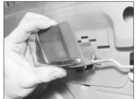
26.4 Withdraw the handle from the door
