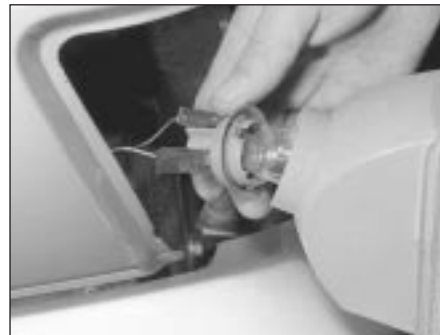
5.14 Withdraw the lens assembly and remove the bulbholder
