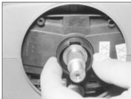
18.8 Position the direction indicator cancelling bush with the slot pointing upwards
