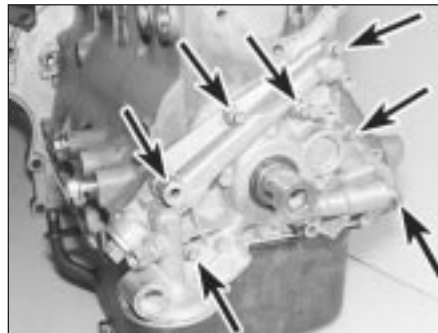
14.8 Oil pump housing retaining bolts (arrowed)
