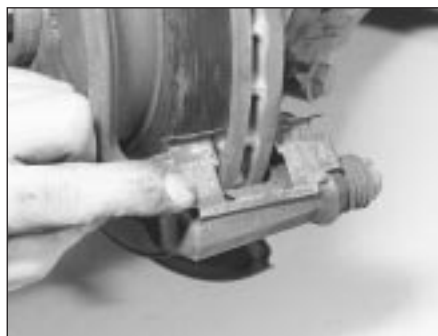
3.4c ... and lower anti-rattle shim
