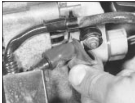
17.12 Pull back the rubber cap and unscrew the main terminal nut
