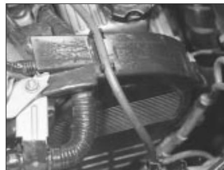
16.27 On V6 engines, remove the pulley covers over the top of the engine ...
