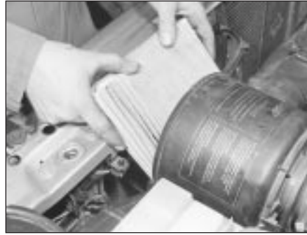
12.1b . . . and element on 4-cylinder engines with single-point fuel injection
