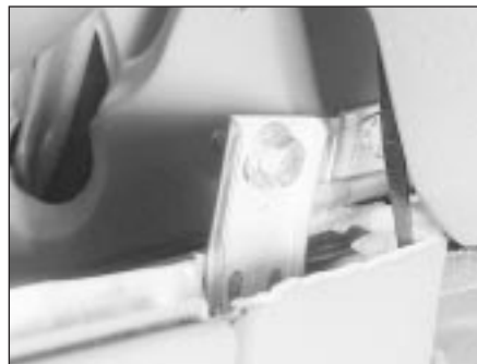
48.14 Undo the bolt at the facia lower end
