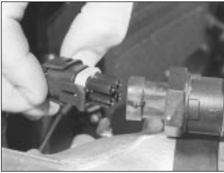
11.14 Disconnect the stepper motor wiring multiplug
