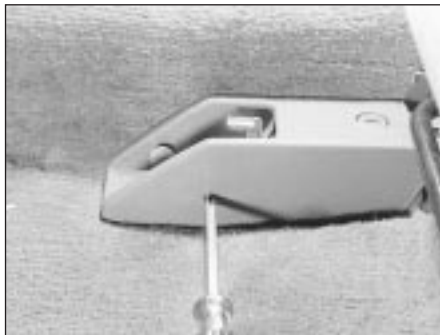
11.2 Undo the release lever control cover retaining screws
