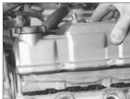
5.5 Lifting off the front camshaft cover
