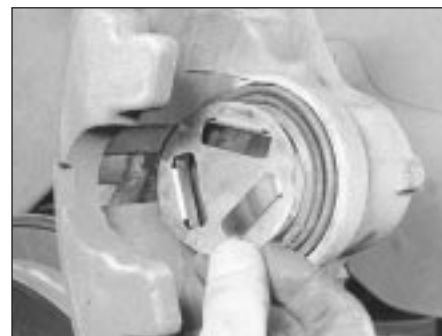
3.5 Remove the heat shield from the caliper piston
