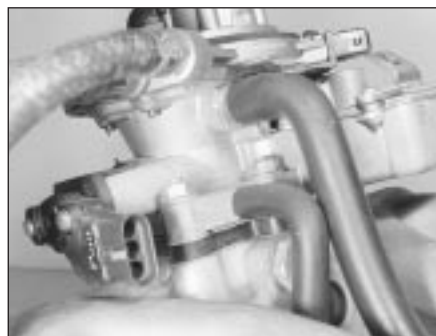
12.35 Breather hose attachments at the throttle body
