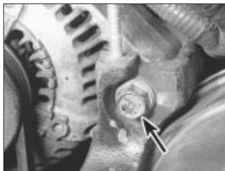
17.10a V6 engine alternator side pivot bolt (arrowed) . . .
