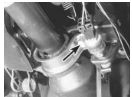
21.11 Steering column lower mounting bolt (arrowed)
