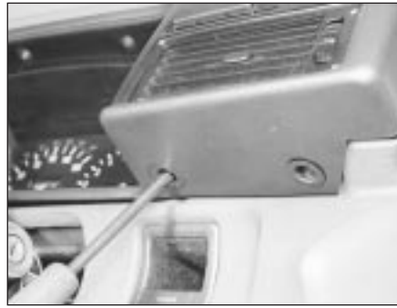
9.6 . . . and the two screws each side at the bottom
