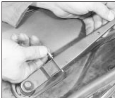
15.1 Insert a pop-rivet through the hole in the wiper arm
