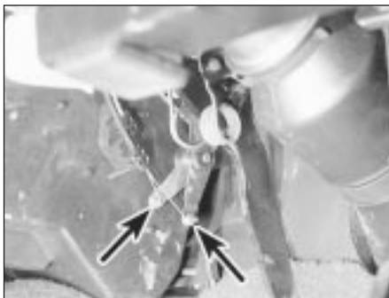
48.3 Release the heater cables at the heater (arrowed)
