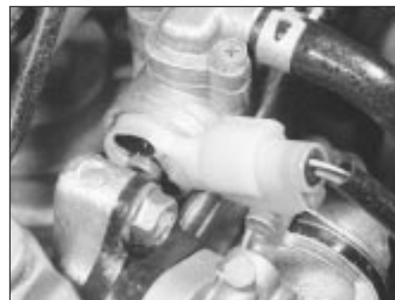
12.31 Disconnect the wiring multiplug from the idle control valve
