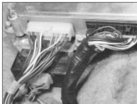
12.80 Disconnect the ECU wiring multiplugs
