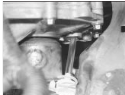
20.2 Topping up the manual transmission oil
