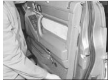
21.14 Withdraw the panel from the door
