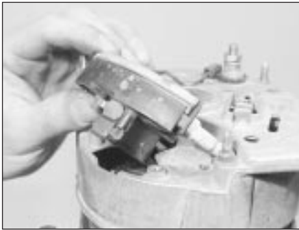
18.3a Withdraw the regulator and brushbox . . .
