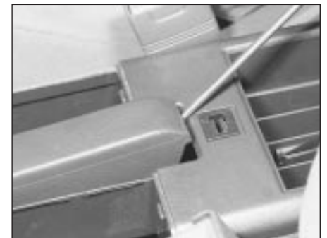
17.6a Prise up the rear of the handbrake lever trim cover . . .
