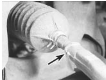
22.2 Steering track rod retaining locknut (arrowed)
