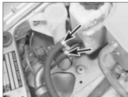
4.28 Disconnect the two power steering hoses at the fluid reservoir
