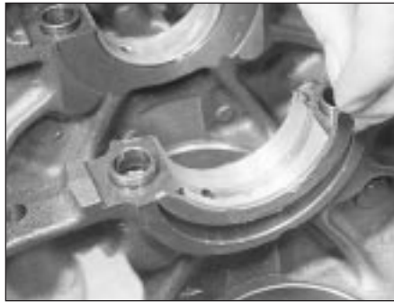
21.5 Fitting the crankshaft thrustwashers
