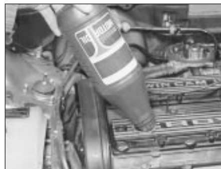
3.6a Topping up the engine oil on 4-cylinder engines . . .
