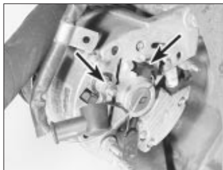
17.4 Typical alternator wiring connections (arrowed) on 4-cylinder engines
