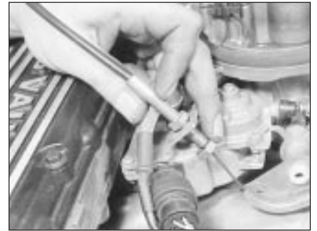
3.2 Undo the accelerator cable locknut ...
