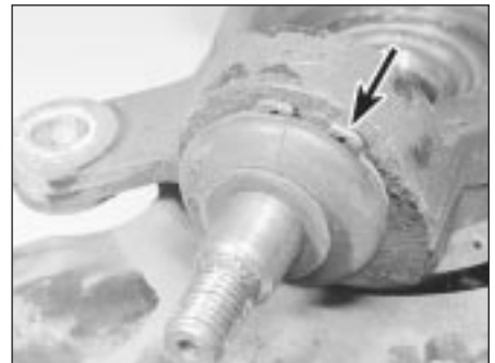
4.2 Balljoint retaining circlip (arrowed)
