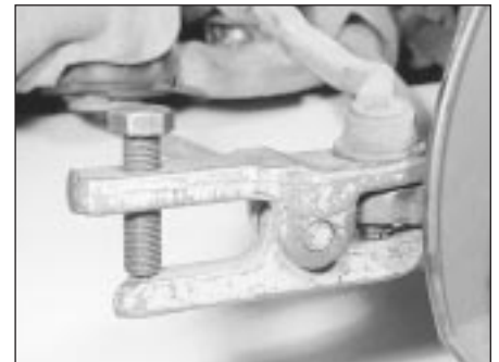
22.4 Using a universal balljoint separator tool to release the track rod balljoint
