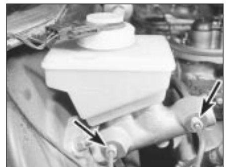
11.4 Unscrew the two brake pipe unions (arrowed) at the master cylinder
